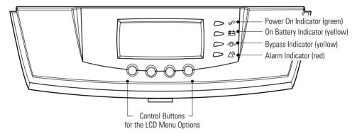
Figure 28. Powerware 9155 Control Panel
