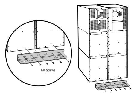
Figure 24. Stabilizing Bracket with Two Cabinets
