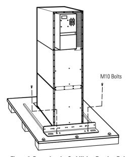
Figure 2. Removing the Stabilizing Bracket Bolts
