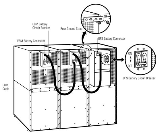
Figure 26. Typical EBM Installation (2-High Cabinets Shown)
