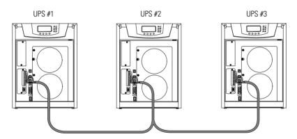
Figure 19. CAN Bridge Card Wiring
