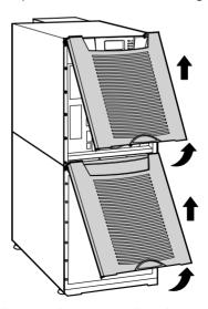
Figure 17. Removing the Front Covers
