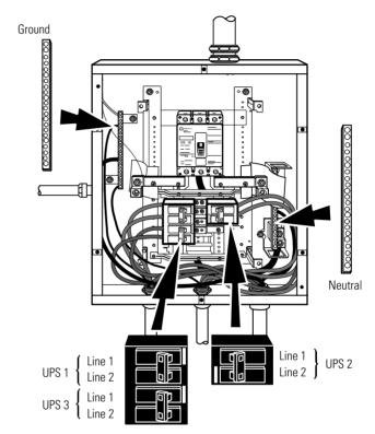
Figure 11. UPS Output to Parallel Tie Cabinet Wiring
