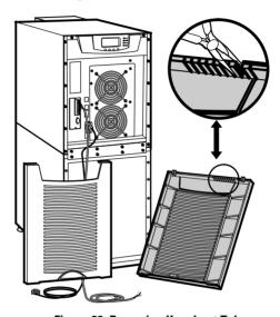
Figure 20. Removing Knockout Tabs
