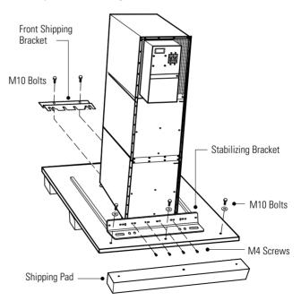
Figure 3. Removing the Brackets and Shipping Pad
