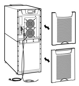
Figure 21. Reinstalling the Front Covers
