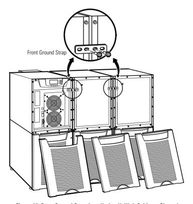
Figure 27. Front Ground Strap Installation (2-High Cabinets Shown)
