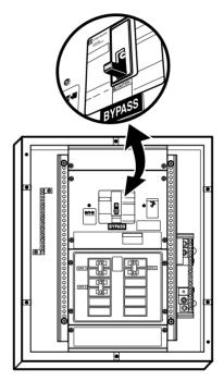
Figure 8. Parallel Bypass Breaker
