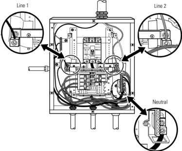
**Figure 12. Load Connections**
