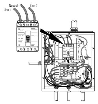
**16.** Wire the AC input to the bypass breaker (see Figure 13).
