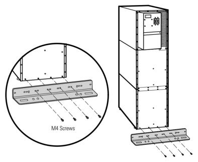
Figure 23. Stabilizing Bracket with One Cabinet
