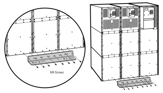
Figure 25. Stabilizing Bracket with Three Cabinets
