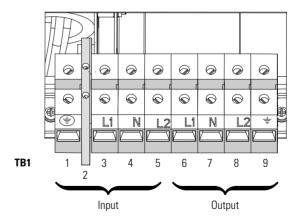
Figure 10. UPS Terminal Block
