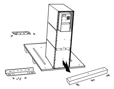
Figure 4. Unloading the Cabinet
